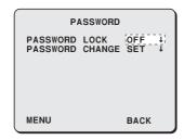
Use the joystick lever (↑↓) to select [PASSWORD LOCK] – "OFF ↓", and press the [ENTER] button.
